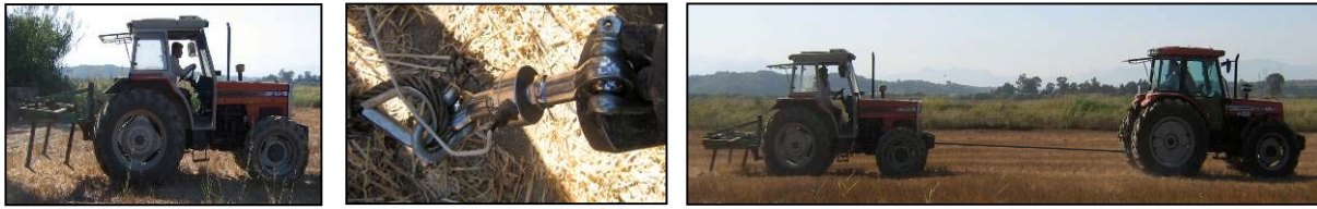
Figure 2. Subsoiler-tractor connections, dynamometer and experimental study
